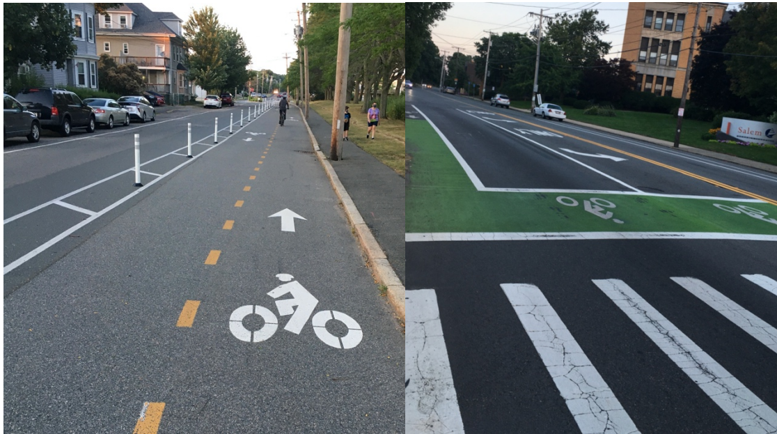
Examples of new bicycle infrastructure in Salem—a Two-Way Protected Bike Lane on Derby St. and a Bike Box at an intersection on Lafayette St.
